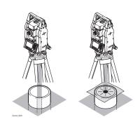
Under some circumstances the laser dot is not visible, for example over pipes. In this case, using a transparent plate enables the laser dot to be seen and then easily aligned to the center of the pipe.
