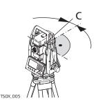
The line-of-sight error (c) is the deviation from the perpendicular between the tilting axis and line of sight. This could be eliminated by measuring in both faces.
