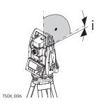
With a horizontal line of sight the vertical circle reading should be exactly  $90^{\circ}(100 \text{ gon})$ . The deviation from this value is termed the Vertical index error (i).
