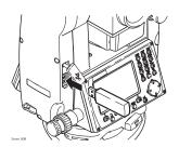
Lift the lid covering the USB host port on the instrument.
