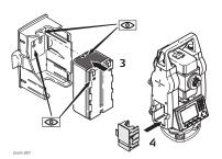
Insert the new battery into the battery holder (3), ensuring that the contacts are facing outward. The battery should click into position.
