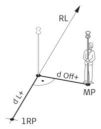
RL Reference line 1RP Start point MΡ Measured point Longitudinal offset dL dOff Parallel offset
