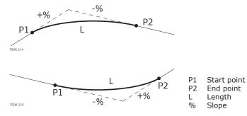
Horizontal and vertical geometry elements combined
