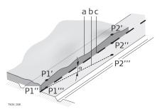
Any project point P1 has E, N and Z coordinates in a determined coordinate system and has three positions.
