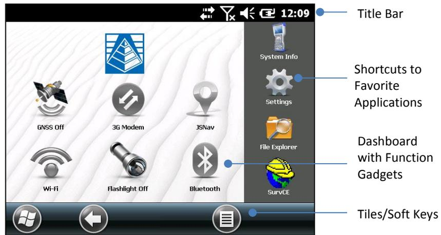
This screen is automatically shown when the Surveyor2 is turned on. You can get to it from any other screen by pressing and releasing the Home screen
