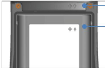
Line up the + and - symbols on the case and the battery pack as shown
