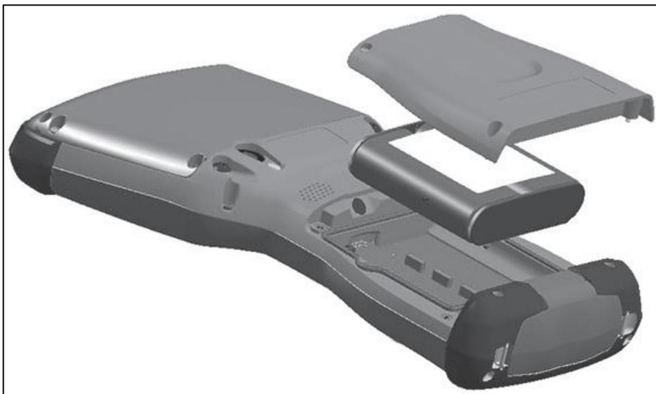
2. If you are using a micro SD card for additional memory or a SIM card with the 3G Data Modem (optional only included on the Cell models of the Surveyor2), you can install them
