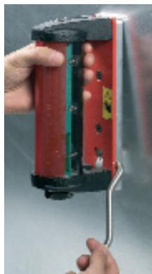
Before placing the receiver on the excavator arm, pull down on the release lever.
