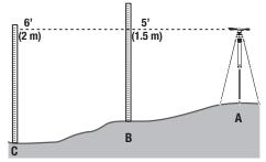
The above illustration shows how exactly we can check the difference in height (or elevation) between two points. If the rod reading at **B** is 5 ft (1.5 m) and the reading at **C** is 6 ft (2 m), we know that point **B** is 1 ft (0.3 m) higher than point **C**. Using the
