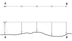
To align the intermediate points, direct the person with the leveling rod to the right or left until the rod coincides with the vertical cross hair. It is important not to move the instrument during operation.
