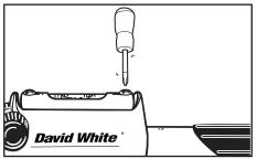
With the bubble level adjustment screw **17** facing to the right of the bubble and with telescope directly in line with two of the three leveling screws, note to which side the bubble is off.
