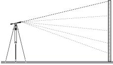
To establish vertical lines and planes, first level the instrument, then release the locking levers which hold the telescope in the level position.
